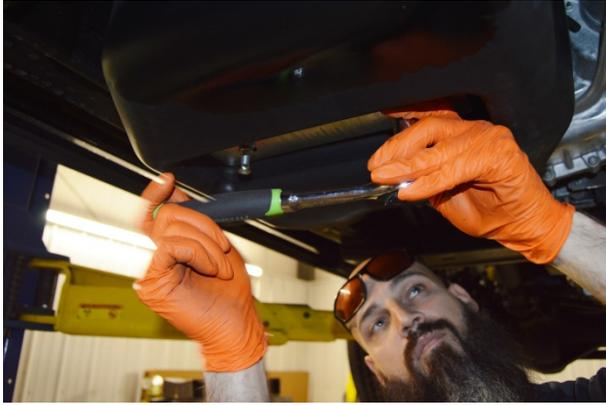
(Fig. 16) Tighten Front Support Assembly to 15 lb.-ft.
