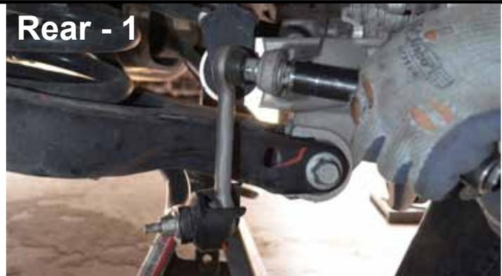
Remove sway bar end link from knuckle on both sides of vehicle.
