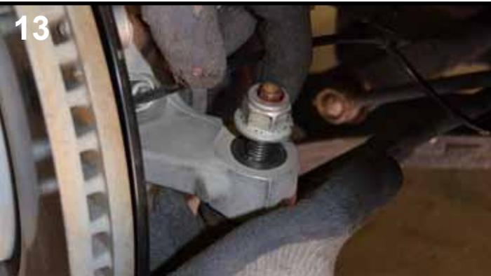
Re-tighten the axle nut, reinstall the tie rod (above) and the ABS/brake lines.
