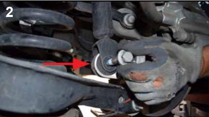
Remove the lower shock mounting bolt.
