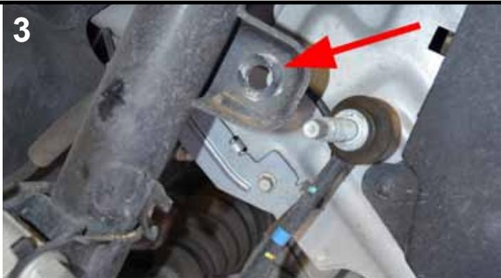
Disconnect sway bar end link from strut.
