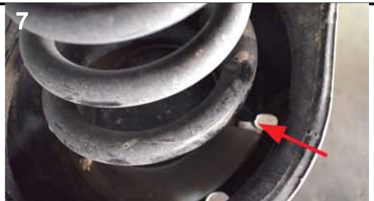
Reinstall coil spring, making sure the bottom of the spring lines up correctly in the LCA, see image.
