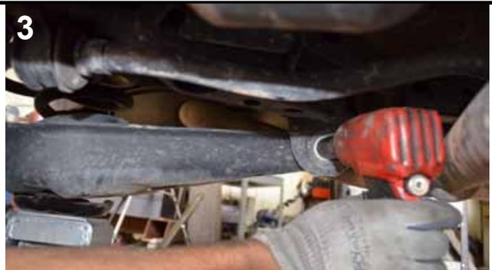
Loosen, but do not remove, the lower control arm (LCA) bolt at the frame.
