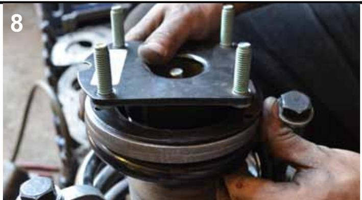
Install spring preload spacers between strut mount and rubber isolator. Reattach strut mount to strut.
