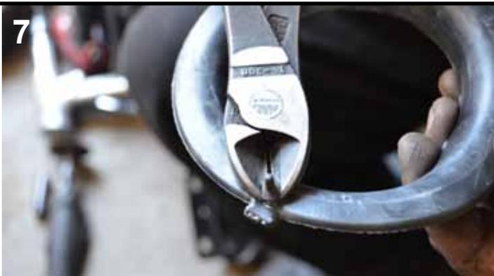
Using a spring compressor remove upper strut mount from strut. Cut off nipples from rubber isolator.
