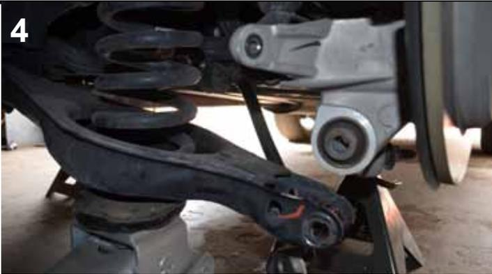
Support the LCA with a floor jack and remove the mounting bolt at the steering knuckle. Carefully lower LCA and remove the coil spring.
