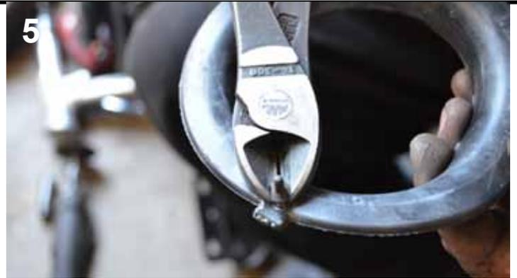
Cut off both nipples from the rubber spring isolator.
