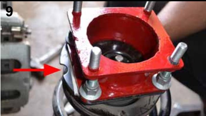
Install the Traxda spacer on strut using factory hardware. Reinstall, making sure the curved edge of strut mount faces the engine, and the notched edge of the spacer faces away from the engine.
