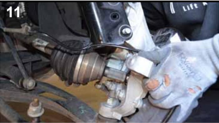
Reinstall lower strut mounting bolts while guiding axle through the spindle. Tighten all strut nuts fully, upper and lower.
