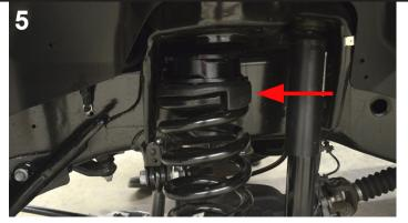
Install coil springs and Spacer back into vehicle, and raise the axle while guiding coil springs into place. Make sure the spring is orientated the same way as when it was removed.
