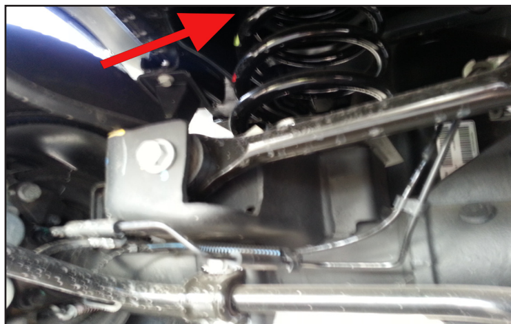
Raise rear of vehicle and support with jackstands at frame on both sides. Remove wheels, support axle on one side and remove the lower shock mounting bolt.
