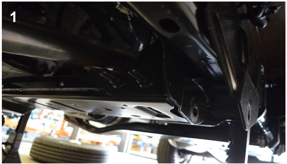
Remove Radius Arm bolts and lower arm. Remove two nuts on crossmember.
