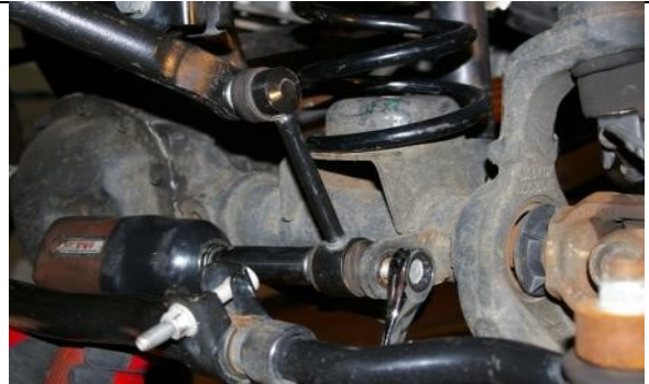
Remove dr./pass. lower front sway bar end links. These will be replaced with the factory rear end links later.
