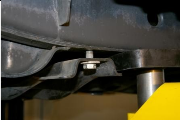
Remove (2) front transfer case skid plate bolts.
