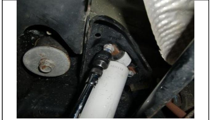
Next, remove rear upper shock bolts.
