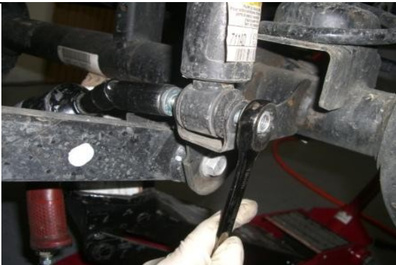
Disconnect and remove front lower shock hardware.
