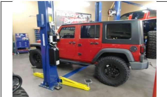
Reinstall wheels and tires and lower vehicle to ground.
