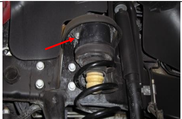
Bolt-in spacers, install OE isolator, then bump stops & springs
