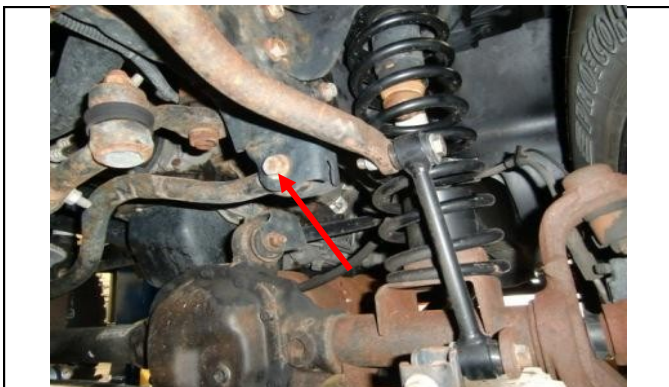
Reconnect front upper track bar with OE hardware and
