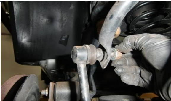
Disconnect rear sway bar end links. Save rear links as these will be used on the front sway bar.
