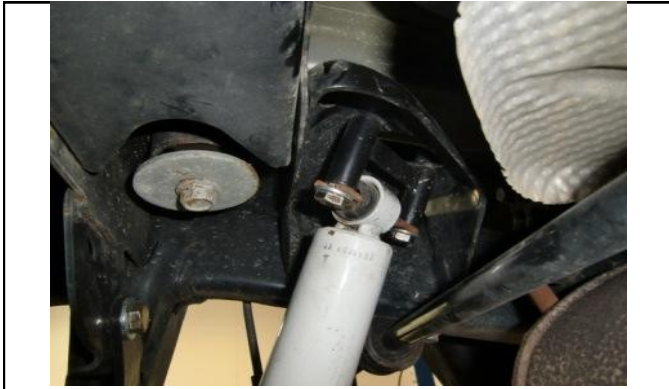
Install upper shock extensions with provided hardware.
