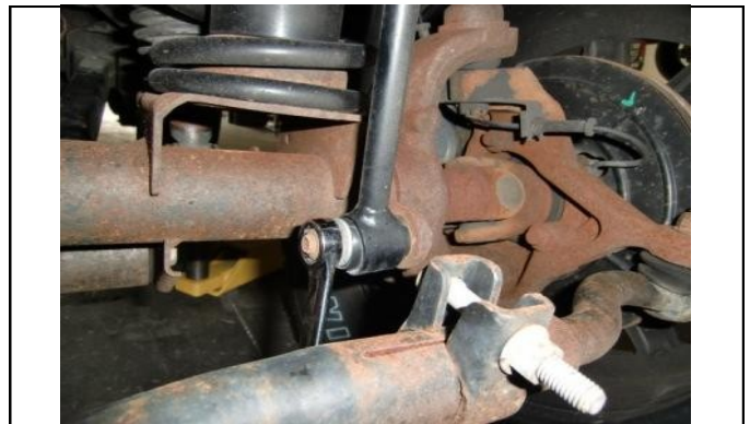
Attach factory rear end links to front sway bar.
