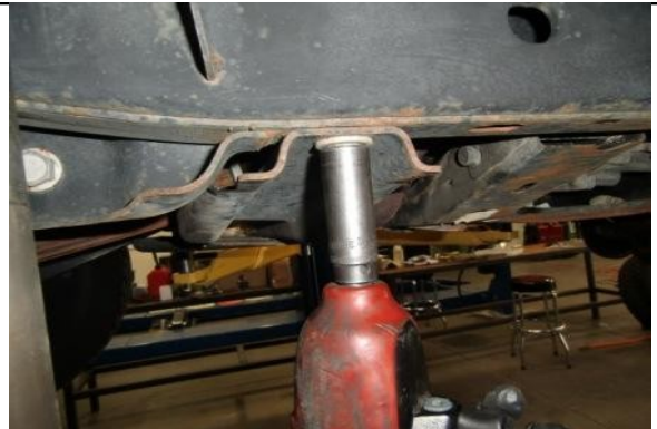
Reinstall front transfer case skid plate bolts.
