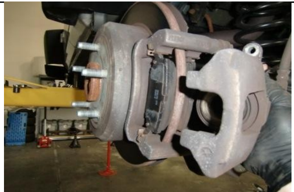
Remove rear brake calipers.
