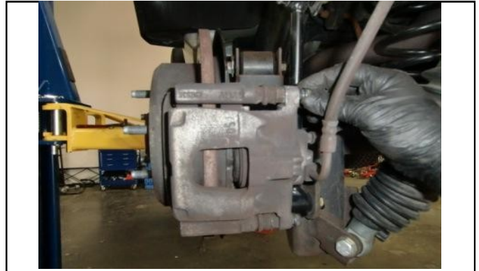
Reattach rear brake calipers and tighten to spec.
