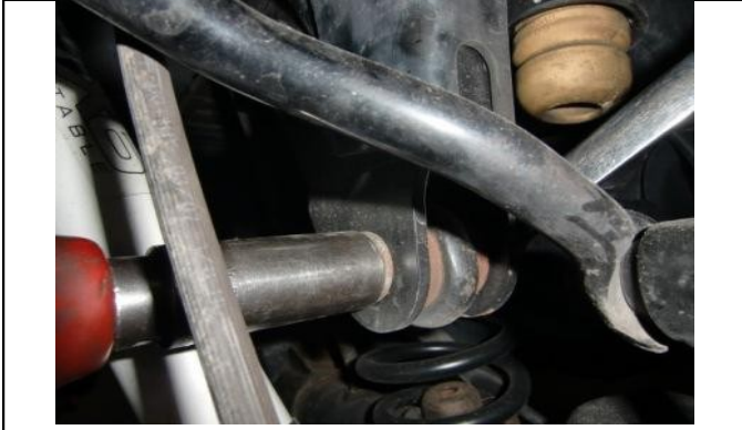
Slightly lift rear axle and remove upper track bar bolt.
