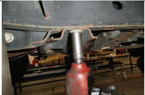
Reinstall front transfer case skid plate bolts.
