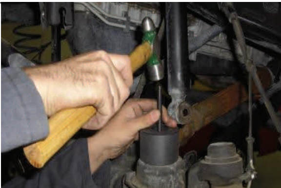
Center, mark and drill 11/32 hole for self tapping bolt.
