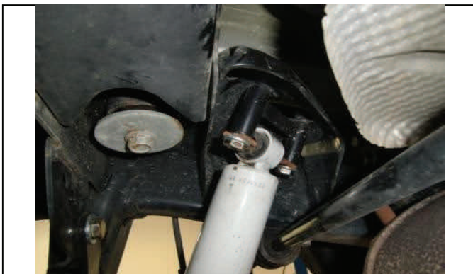
Install upper shock extensions with provided hardware.
