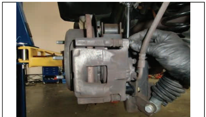
Reinstall rear brake calipers and torque to spec.
