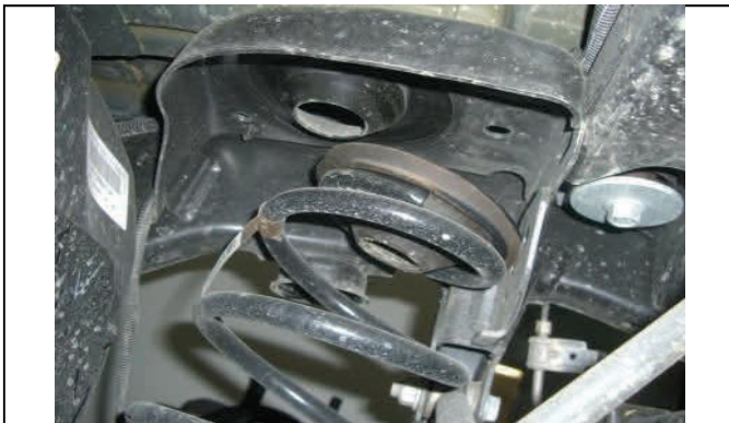
Carefully lower rear axle and remove rear coil springs.
