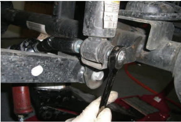
Disconnect and remove front lower shock hardware.
