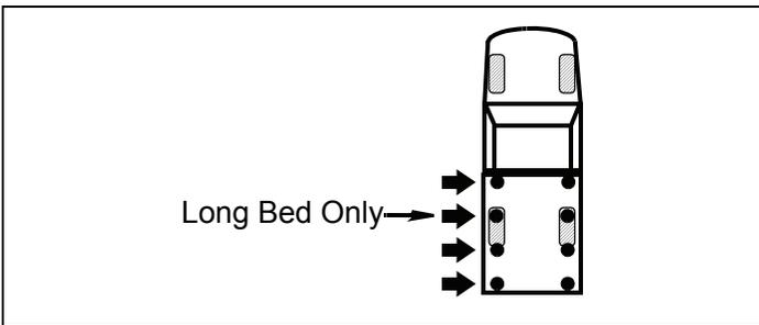
12. Remove bed mounting bolts from passenger side only.
