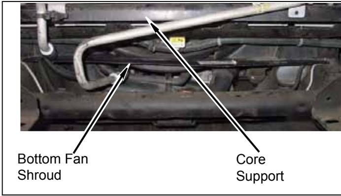
e. Mark & Drill two holes in upper fan shroud bracket using computer module as a template. Install computer module on upper fan shroud with two pop-up clips.
