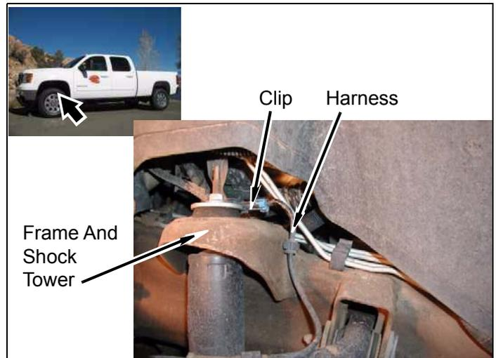
c. Remove two clips and harness from cover and inner fender.
