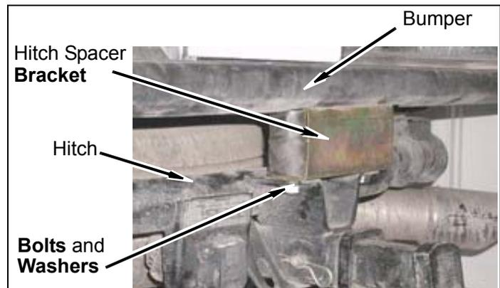
r. Adjust bumper to bed clearance using measurements taken earlier and tighten hitch bolts first then remaining bolts and nuts to 55 lb-ft.
