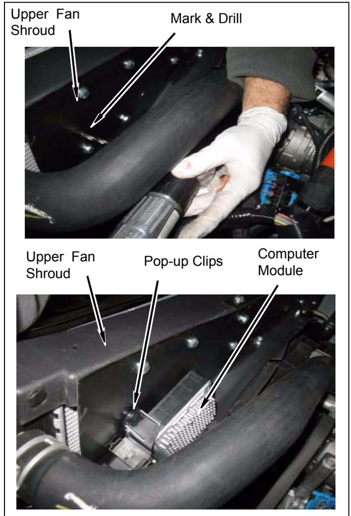
c. Install upper fan shroud assembly on core support with two bolts. Do not tighten.
