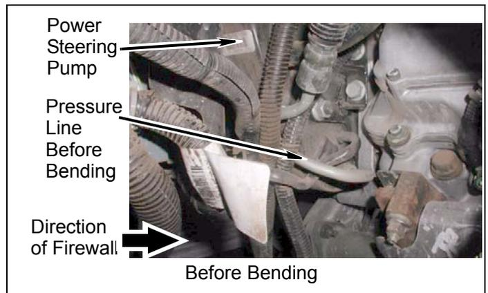
7. Wiring harnesses and power steering drivers side
