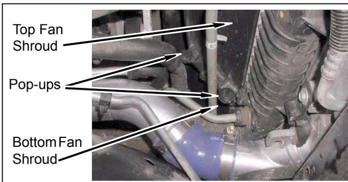
f. Install three *kit lower fan shroud plates* with two *kit bolts* (1/4" x 3/4"), four *kit washers* (1/4" SAE), and two *kit nuts* (1/4" nylock).
