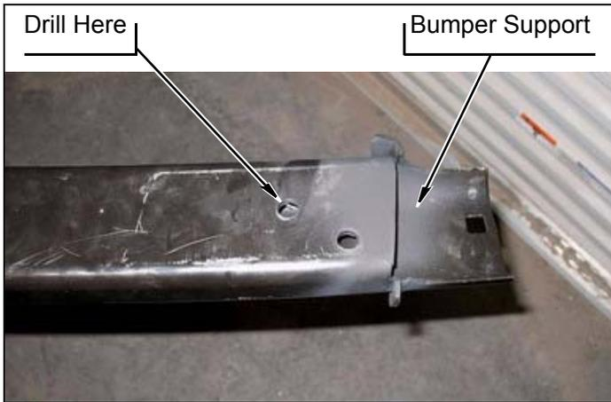
l. Install bumper support onto two *kit brackets* (bumper, rear) with four *kit bolts* (1/2"-13 x 3"), eight *kit washers* (1/2" SAE) and four *kit nuts* (1/2"-13 Stover). DO NOT TIGHTEN.
