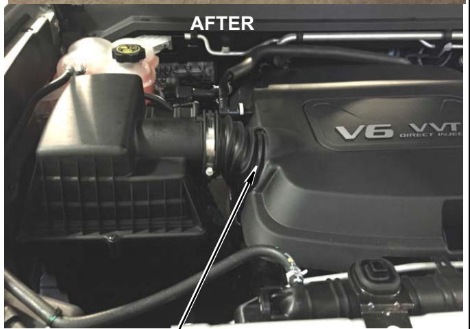
Air-Intake Box Cut and Installed
