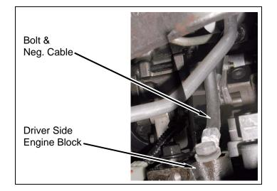
b. Install *kit* **bracket** (angled) onto engine with bolt. DO NOT TIGHTEN.
