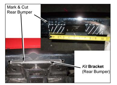
e. Apply small amount of kit Loctite® onto threads of two *kit* **bolts** (7/16" x 1-1/2") and install rear bumper onto *kit* **bracket** (rear bumper, middle) with two *kit* **bolts** (7/16" x 1-1/2"), four *kit* **washers** (7/16" USS), and two *kit* **nuts** (7/16" Nylock). DO NOT TIGHTEN.
