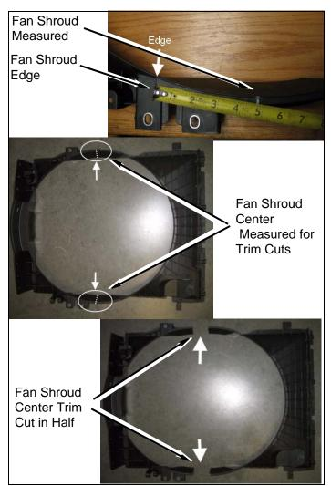
d. Separate both halves of the fan shroud on a flat and level surface. (**Note**: Allow for lower edge of fan shroud to over hang your flat surface; this will allow the shroud to sit level on a table or work bench.) e. Separate fan shroud so that each side is equally "gapped" to **3**"; extending the over all length of the fan shroud by **3**".
