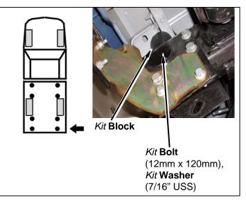
c. Install *kit* **blocks** onto two (or three) other frame mounts.
