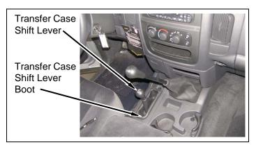
d. Remove cup holder inserts, three screws, and center console from floor.
