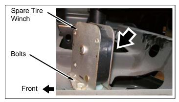
b. Install *kit* **bracket** (spare tire winch) onto crossmember with factory driver side bolt. DO NOT TIGHTEN.
