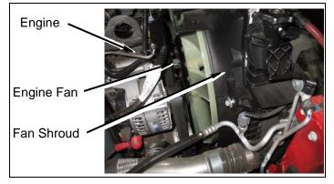
c. Remove fan shroud and engine fan as assembly from engine compartment.
