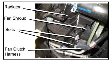
b. Using proper tool; remove fan from engine water pump.
