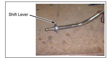
e. Install two plastic shift tabs, plastic ball, shim, and mounting plate onto shift lever.
