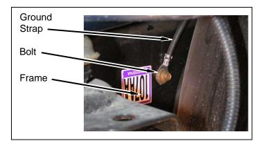
3. Remove nut and ground strap from stud on lower driver side firewall.
