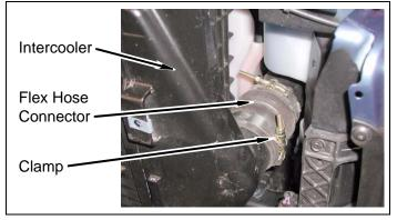
d. Install intercooler onto upper core support with two bolts..
