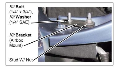
Install airbox onto *kit* brackets (airbox) and *kit* bracket (airbox mount) with *kit* bolt (1/4" x 3/4"), two *kit* washers (1/4" SAE), and *kit* nut (1/4" Nylock). TIGHTEN all hardware.
