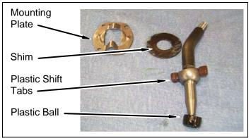
b. Scribe a line along side of transmission shift lever (below lowest bend). Measure diameter of shift lever (below lowest bend). Cut lever into two pieces and deburr as necessary.
