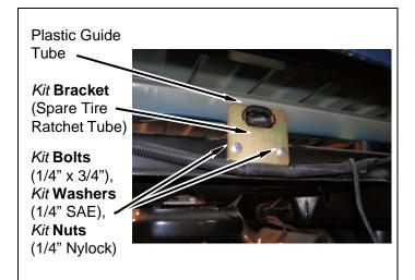
i. Install ratchet tube onto spare tire winch with retaining clip.
