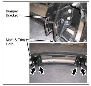
b. Apply small amount of *kit* **Loctite**® onto threads of factory front bumper bolts.
