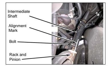
Remove bolt and intermediate shaft from rack С and pinion. Slide intermediate shaft up to separate from rack and pinion.
