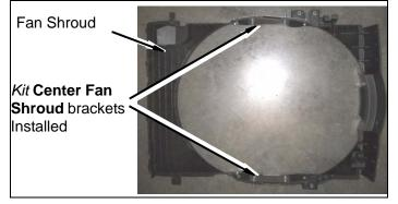
j. Carefully reinstall engine fan & fan shroud back into lower locking tabs and engine fan clutch back onto engine water pump pulley with correct tooling.
