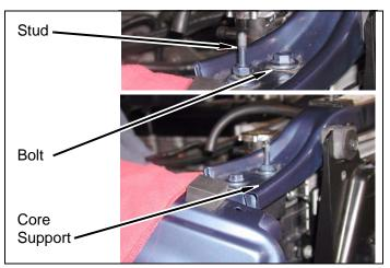
b. Install stud and bolt into passenger side core support in opposite locations.
