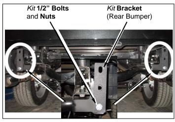
d. Measure, Mark & Cut rear bumper center section to clearance *kit* **bumper** (center) **bracket**.
