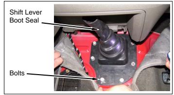
h. Remove two nuts and manual transmission shift lever from shift tower.
