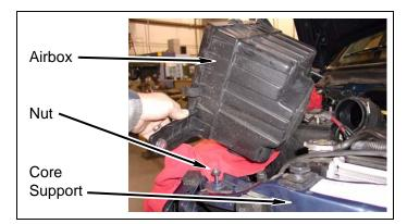
Remove two push clip standoffs and AC line C. from passenger side core support.
