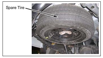
b. Remove retaining clip and ratchet tube from spare tire winch mechanism.
