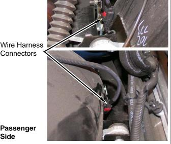
4. Remove two push clips and block heater cord from passenger side frame, if equipped.
