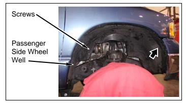
t. Install brake sensor wiring harness push clips onto passenger and driver side wheel wells.
