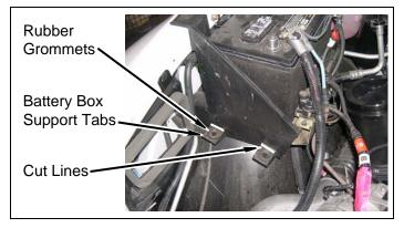
Mark two cut lines on battery box support tabs. Cut support tabs from battery box along lines. Where support tabs were cut from battery box, ensure smooth surface. Grind or sand, if necessary.
