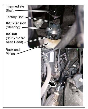
b. Install intermediate shaft on *kit* **extension** (steering), ensuring marks on intermediate shaft and rack and pinion are aligned.
