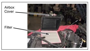
b. Remove nut and airbox from core support and battery box.
