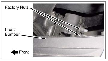
c. Remove two bolts from top of intercooler and core support.
