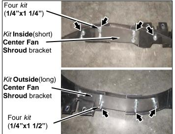
**Note**: Be sure to install all kit(1/4") hardware from inside to outside of kit fan shroud brackets. Doing so will eliminate the chance of kit hardware contacting the engine fan after shroud is reinstalled into vehicle.
