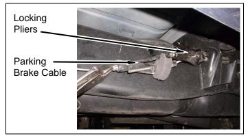
b. Use expanding pliers and disconnect parking brake cable from junction.
