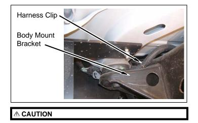
Some slight bending of the brake lines is required to align brackets with holes in frame rail. Use caution when bending brake line.
