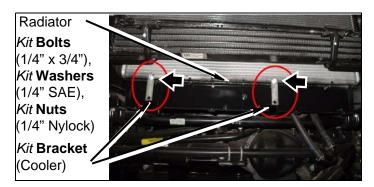
b. Install transmission cooler onto two *kit* **brackets** (cooler) with two *kit* **bolts** (1/4" x 3/4"), four *kit* **washers** (1/4" SAE), and two *kit* **nuts** (1/4" Nylock).
