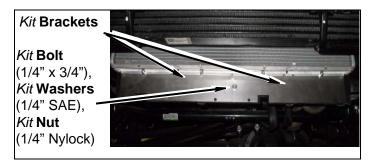
m. Install both *kit* **lower fan shroud brackets** into lower radiator pocket. Attach kit brackets with four *kit* **bolts**(1/4"x3/4"), **washers** & **nuts** onto back side of lower radiator.
