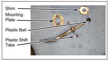
f. Install shift lever onto shift tower with four Torx bolts.
