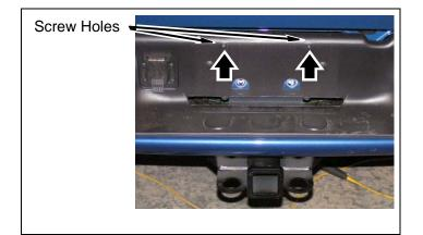
c. Remove two bolts from center of bumper.
