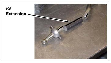
d. Grind welded surfaces smooth in order to install mounting plate and shim to shift lever.
