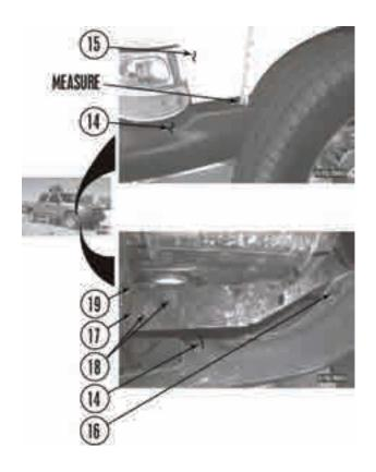
d. Remove four bolts (20) and front bumper (14) from frame (19).
