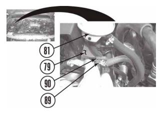
f. Remove wire harness (91) from clip (92) on passenger side wheel well (79) behind power steering reservoir (81).
