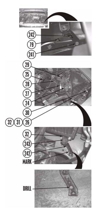
f. Install bracket (242) on lower air cleaner housing (32) and driver side wheel well (79) with two bolts with captive washers (241 and 243).
