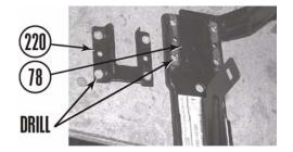
b. Install power steering slotted bracket (220) on kit power steering Z bracket (221) and kit power steering C bracket (222) with four kit 1/4" x 1" bolts (216), eight 1/4" SAE washers (217), and four kit 1/4" nylock nuts (218). Install kit 1/4" x 1" bolts as shown.
