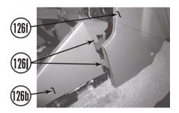
b. Install storage console (126b) on cab (105) with six screws (126i).
