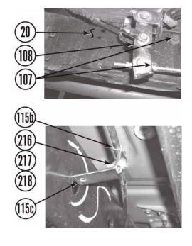
b. Install *kit* bracket (115c) on frame (20) driver side with bolt (115a).
