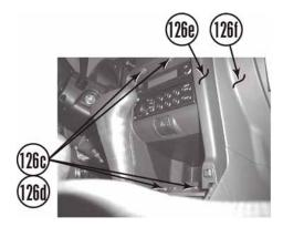
e. Position shift lever console (126a) on storage console (126b) and if applicable, install manual shift knobs (123 and 124) on manual shift levers (125 and 126).
