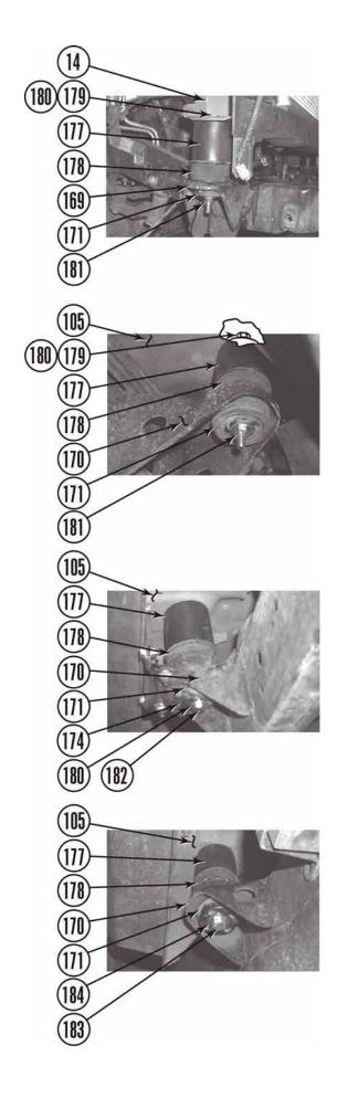
6. Install the bed passenger side spacer blocks.
