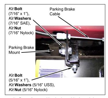
d. Route front parking brake cable through largest hole in *kit* **bracket** (parking brake) and connect parking brake cable.
