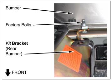
f. Align rear bumper to previous bed-to-bumper measurements. TIGHTEN all hardware.
