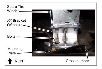
d. Install spare tire winch onto *kit* **bracket** (winch) with two *kit* **bolts** (3/8" x 1"), four *kit* **washers** (3/8" USS), and two *kit* **nuts** (3/8" Nylock).
