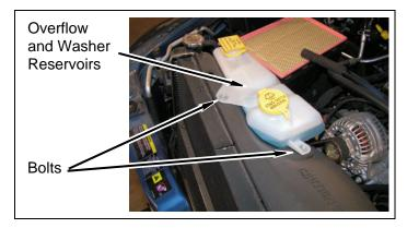
b. Disconnect and cap off overflow and washer hoses.
