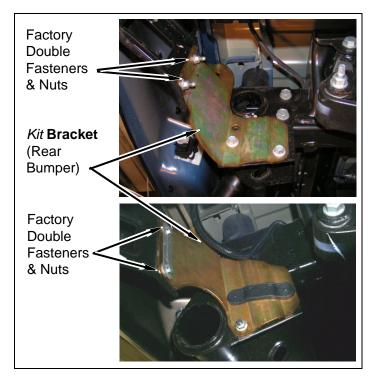
d. Install rear bumper onto kit bracket (rear bumper, middle) with two kit bolts (7/16" x 1-1/2"), four kit washers (7/16" USS) and two kit nuts (7/16" Nylock). DO NOT TIGHTEN.
