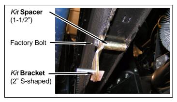
c. Install power steering cooler onto two kit brackets (2" S-shaped) with two kit washers (1/4" SAE) and two kit nuts (1/4"-20 Nylock). DO NOT TIGHTEN.
