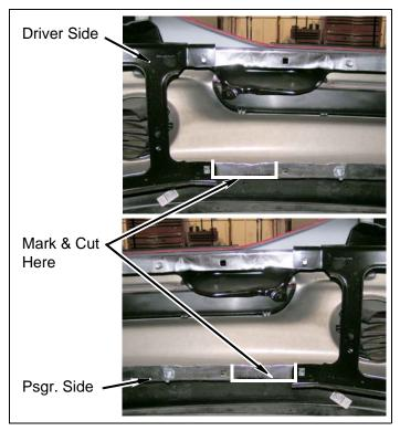
g. Mark and cut driver and passenger side front bumper as shown.
