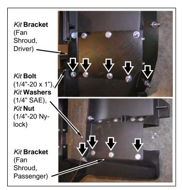
j. Install kit gap guard (fan shroud) inside upper and lower portions of fan shroud. Using kit cover (fan shroud) as a template, mark and drill a 1/4" hole corresponding to each hole on kit cover (fan shroud).
