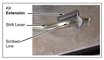
b. Scribe a line along side of kit extension (shift lever). Position kit extension between two pieces of transmission shift lever. Ensure scribed lines on kit extension and transmission shift lever align. Weld kit extension into place.
