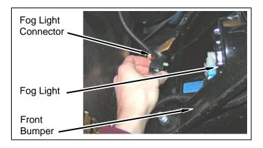
Remove eight nuts and front bumper from frame horns.
