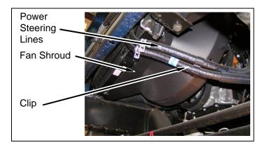
c. Remove two bolts and fan shroud from radiator.
