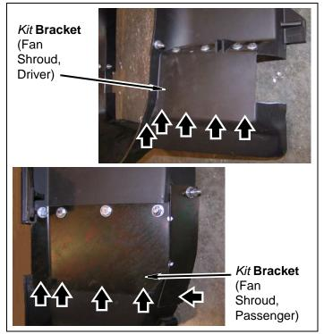
Install kit brackets (fan shroud) onto lower portion of fan shroud with kit bolt (1/4"-20 x 1"), two kit washers (1/4" SAE) and kit nut (1/4"-20 Nylock) at each drilled hole location. Snug, but DO NOT TIGHTEN.
