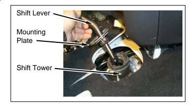
h. Remove two plastic shift tabs, plastic ball, shim and mounting plate from shift lever.
