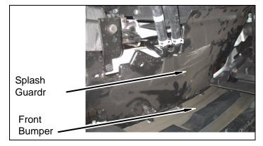
b. Disconnect fog light harness at driver side of front bumper and pull connector off of front bumper, if equipped.
