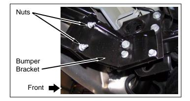
Remove four bolts and bumper brackets from frame.
