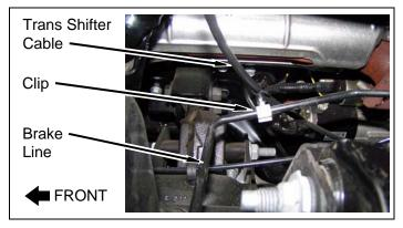
e. **Automatic transmission models:** Remove transmission wire harness from frame mount clip.
