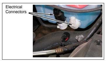
Install radiator overflow and window washer reservoirs onto fan shroud with bolts.
