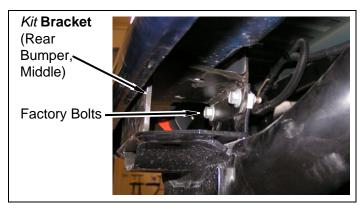
b. Apply a few drops of kit Loctite® to factory bolts. Install kit brackets (rear bumper) onto frame with factory hardware. DO NOT TIGHTEN.
