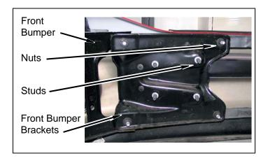
c. Remove two lower crush zones from front bumper.
