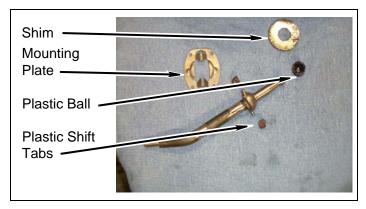
e. Install shift lever onto shift tower with four Torx bolts.
