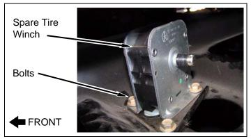
b. Using 9/16" drill bit, drill two mounting holes and remove mounting plate from spare tire winch.
