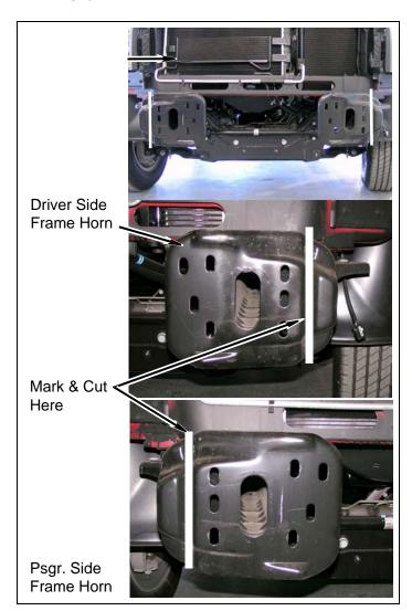
f. Mark and cut driver and passenger side front bumper as shown.
