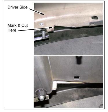
h. Install two lower front crush zones onto front bumper.
