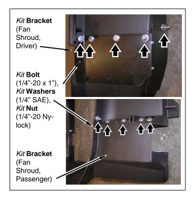
g. Position lower portion of fan shroud with kit brackets (fan shroud) 3" from upper portion of fan shroud as shown.
