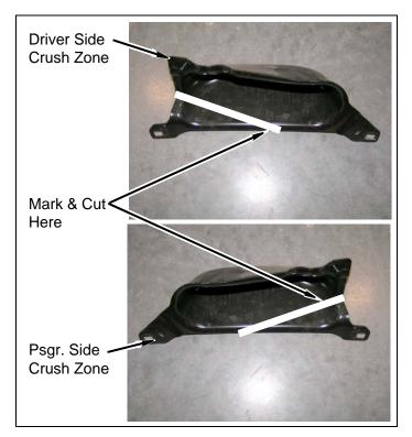
e. Mark and cut two front bumper frame horns as shown.
