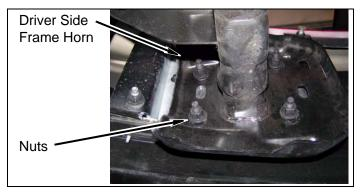
Position front bumper to frame. Ensure both edges of fender well fit on backside of bumper edge.
