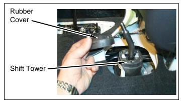
g. Install shift lever boot seal onto floor with six bolts.
