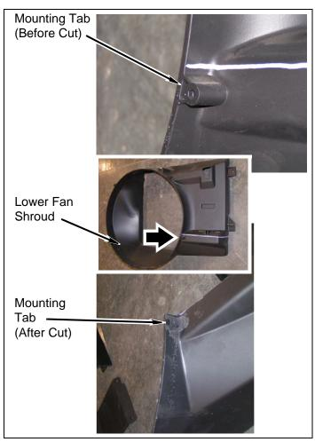
d. Position kit bracket (fan shroud, passenger) on outside upper fan shroud. Using kit bracket (fan shroud, passenger) as a template, mark and drill a 1/4" hole corresponding to each hole on kit bracket (fan shroud, passenger). DO NOT DRILL lower portion of fan shroud at this time.
