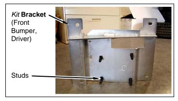
j. Apply a few drops of kit Loctite® onto threads of studs and install two kit brackets (front bumper) onto front bumper with ten nuts. If necessary trim front bumper to fit kit brackets (front bumper).
