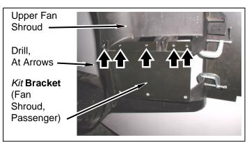
e. Position *kit* **bracket** (fan shroud, driver) on outside upper fan shroud. Using *kit* **bracket** (fan shroud, driver) as a template, mark and drill a 1/4" hole corresponding to each hole on *kit* **bracket** (fan shroud, driver). DO NOT DRILL lower portion of fan shroud at this time.
