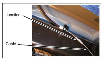
c. Remove parking brake cable from driver side frame mount.
