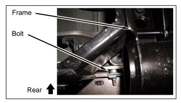
d. Remove two bolts from rear bumper and trailer hitch, if equipped.
