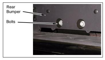
e. Remove four nuts, two double bolt fasteners, and bumper from bumper brackets.
