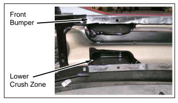
d. Mark and cut driver and passenger side lower front crush zones as shown.
