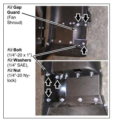
I. Ensure 3" spacing between upper and lower portions of fan shroud. Tighten all hardware.
