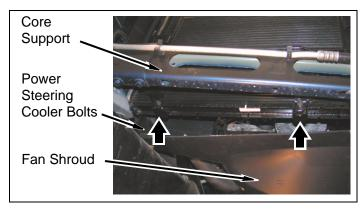
Install fan shroud onto radiator. Ensure fan shroud tabs are seated completely in radiator slots. Install fan shroud to radiator with two factory bolts.
