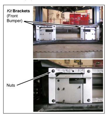
k. Apply a few drops of *kit* **Loctite**® onto threads of studs and install front bumper onto two frame horns with eight nuts. DO NOT TIGHTEN.
