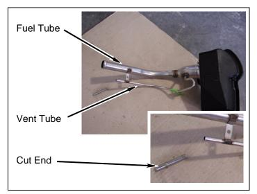
d. Install kit extension (vent, 1/4" x 3") between cut ends of metal vent tube with two kit clamps (#6 hose). DO NOT TIGHTEN.
