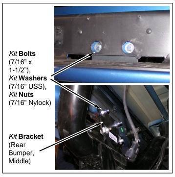
e. Install *kit* **brackets** (rear bumper) onto bumper with two factory bolts. DO NOT TIGHTEN.
