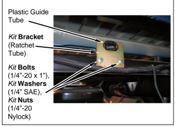
g. Install ratchet tube onto spare tire winch with retaining clip.
