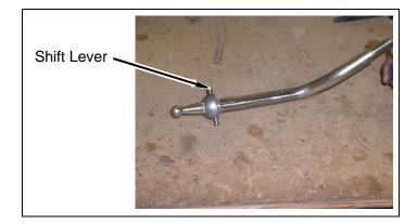
d. Install two plastic shift tabs, plastic ball, shim and mounting plate onto shift lever.
