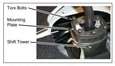
f. Install rubber cover onto shift tower.
