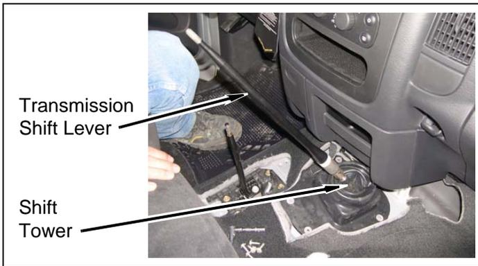
f. Remove six bolts and shift lever boot seal from floor.
