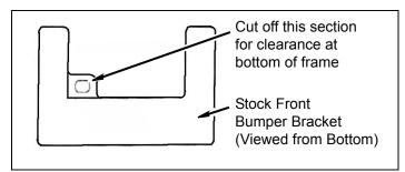
Install stock bumper brackets on rear bumper. Install kit **brackets** on bumper using stock nuts (studs on kit **brackets** should be pointing away from bumper). DO NOT tighten.
