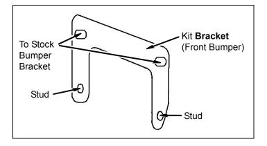
Install rear bumper on vehicle with studs going through original mounting holes. Install a kit **washer** (1/2" USS) and a kit **nut** (1/2" Nylock) on each stud. DO NOT tighten. Adjust bumper using measurements recorded earlier. Tighten all front bumper fasteners.
