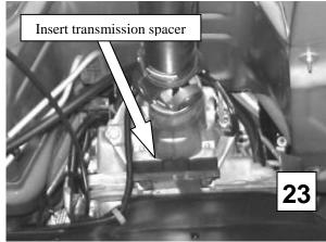
**10a)** Remove the two bolts from the isolator to the transmission, lift and insert the spacer, install the two supplied 10mm bolts thru the spacer and back into the transmission.
