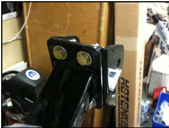
Mock-up shown with Hotchkis leaf spring mount
