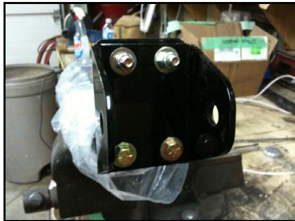
Mock-up shown with Hotchkis leaf spring mount
