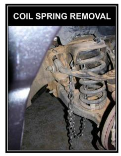
then out the lower control arm. Fasten the chain back to itself leaving only enough slack to allow the coil to unload.
