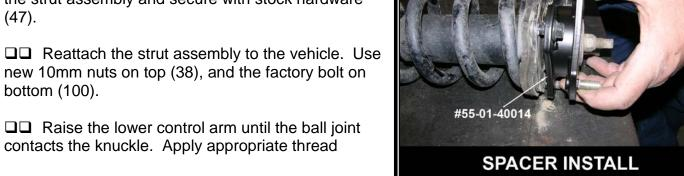
locking compound then install the ball joint-to-knuckle bolts (48).
