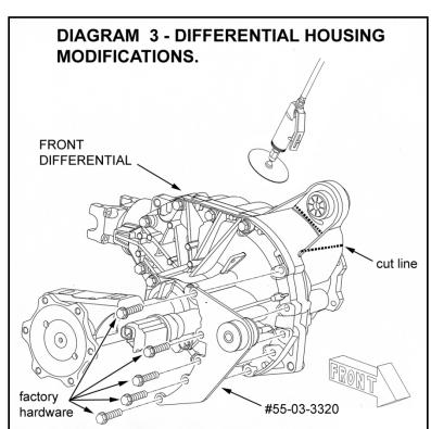
□ [DIAGRAM 3] Remove the factory bolts on the differential and attach the "03" bracket to the housing as shown. Re-install the bolts and tighten (35).
