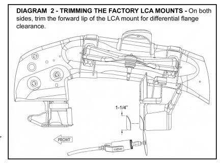
□□ [DIAGRAM 2] Trim the forward lip on both the driver and passenger side lower control arm mounts as shown for proper differential flange clearance.
