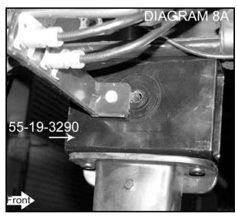
applications, a little more length is needed. If so, bend the factory bracket down slightly to gain the necessary slack in the hose.
