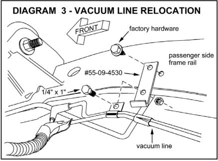
then install the bolt from the outside. Do not tighten at this time.
