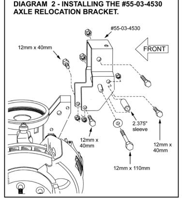
$\Box$  Torque the 110mm bolts (52-55) and the 40mm bolts (73-77).
