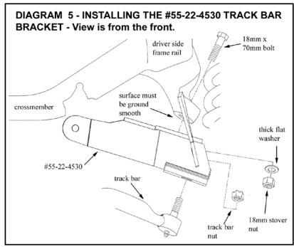
slightly so that the bracket fits flush with the factory track bar mount. Grind as necessary, then check-fit the "22" bracket once again to ensure it fully contacts the factory mount.
