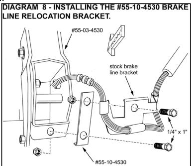
factory bracket slightly to avoid rubbing against the bolt heads.
