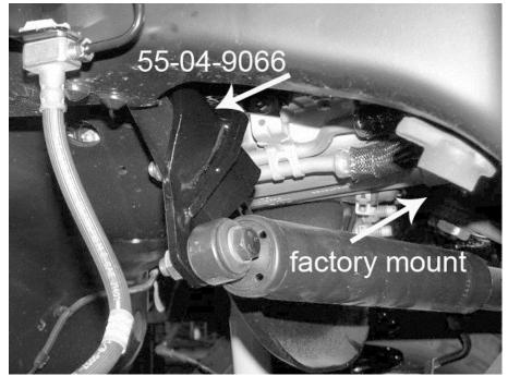
front axle via a bracket located in front of the coil spring's lower seat. Unplug the vacuum line where it passes through this bracket then unbolt the bracket from the axle.
