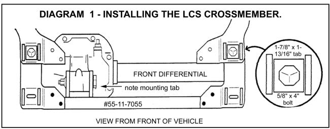
The 1-7/8 " x 1-13/16" tabs are used as locking washers for the 5/8" x 4" bolts that attach the Superlift crossmembers-to-frame pillars. It is not unusual for the frame pillars to be bent somewhat, causing misalignment. If you experience this, and mis-alignment is no more than 1/4", trim the tabs' width until they seat properly. If more than 1/4" mis-alignment exists, contact Superlift before proceeding.
