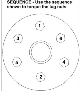
**DIAGRAM 6 - LUG NUT TORQUE**
