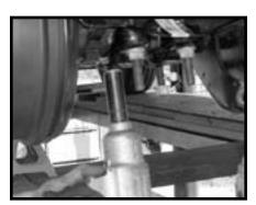
Remove the u-bolts and spring plates.
