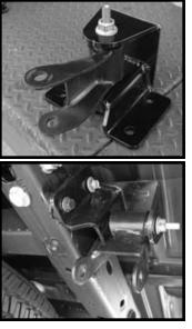
Place the new upper axle plates on top of the axle, align pin with hole on axle. Install the 5/8" bolts provided with one flat washers on top of the upper plate and one on the bottom of the axle locator. Check pinion angle.
