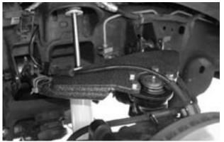
Replacing factory slotted alignment cams on the forward upper mount with cam lock plates. **DO NOT OVER TIGHTEN 40FT lbs max**
