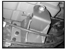
The hangers have 3 holes to attach the leaf spring. This will give some adjustment to the drop. The top hole will give the most drop. It may be easier to bolt the spring to the hanger before bolting hanger to frame.
