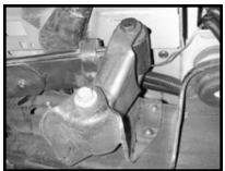
Apply grease to the shackle bushings. Install the shackle with the bushings down and the open side forward. Do not over tighten the spring bolts. The shackle has to move with the flexing of the spring. Check all bolts then test drive.
