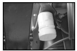
Trim the bumpstop to the point that the truck does not bottom excessively but not so much to over travel the shock absorbers.
