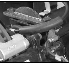
The ideal pinion angle would be perfect alignment when the truck is in motion. With the rear end mounted to leaf springs when power is applied the rear end always moves up slightly. So adjust the pinion just below (-5 degrees) perfect alignment
