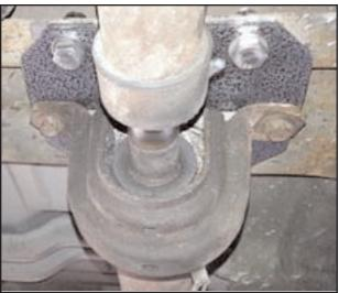
Reinstall the bearing using the original bolts and clips
