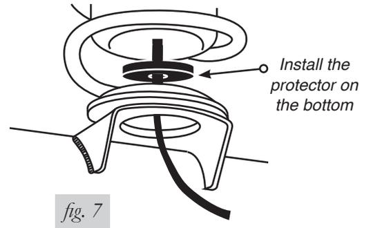
8. When the air spring is completely within the coil, remove the cap and allow the air spring to assume its "as molded" shape.
