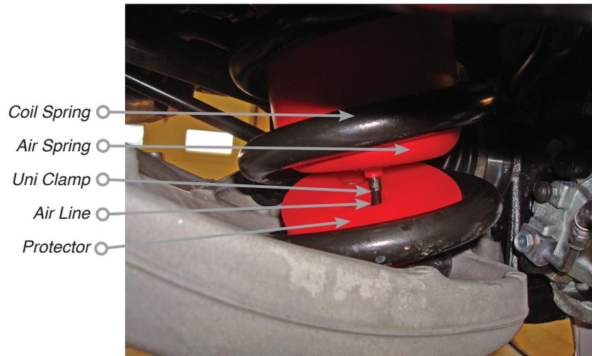
Push air spring to the top and insert protector between the air spring and lower spring seat. Attach hose and uni clamp over barbed stem of air spring.
