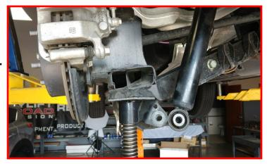
Reinstall the brake line ferrule through the metal mount on the body. Install the spring clip.
