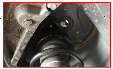
Install the ReadyLIFT strut extension onto the factory top hat using the factory hardware. This is a tight fit to get the bolts into place. The top hat can be rotated to access the bolts. Once all have been started, tighten all down.
