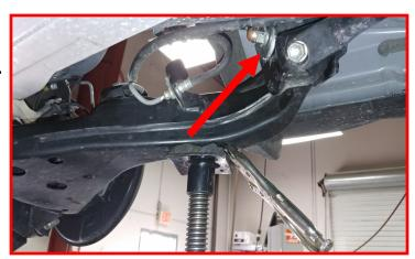
Once the lower control arm is installed into the frame pocket, move the jack to the back of the control arm and raise the arm enough to install the rear shock hardware. Do not tighten at this time.
