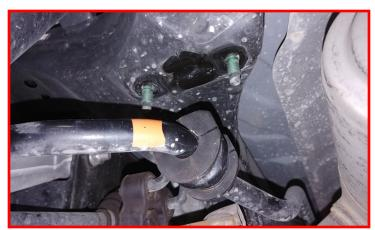
Support the lower control arm with a suitable jack and remove the lower shock hardware.
