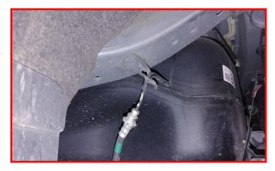
Remove the sway bar from the frame and let hang out of the way.
