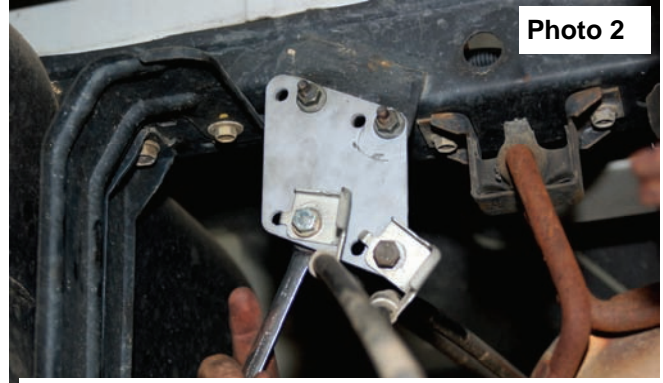
Install Rear E Brake Line Bracket To Rear Frame
