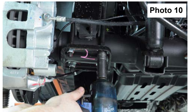
Remove the factory u bolts and hardware.
