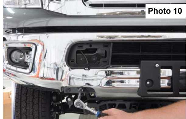
Remove the front bumper mounting bolts.
