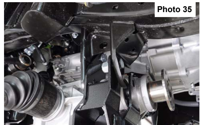
Bolt differential to the rear crossmember.
