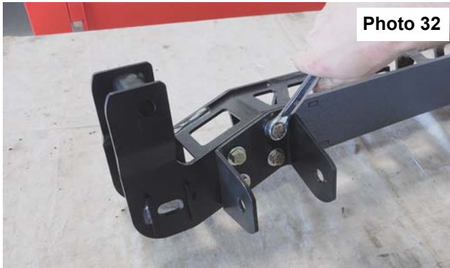
Install differential drop brackets on front crossmember.
