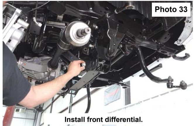
Install differential drop brackets on front crossmember.
