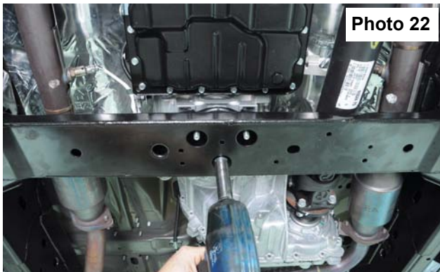
Remove transmission mount nuts.
