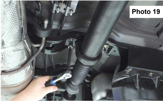
Lower the carrier bearing.
