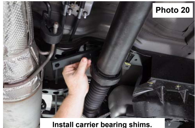
Install carrier bearing shims.
