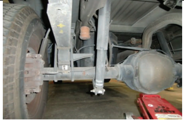
Also support axle by differential
