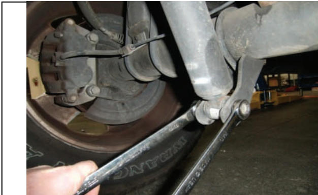
Disconnect lower shock mounting hardware.
