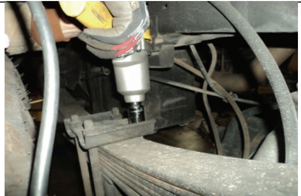
Remove u-bolt nuts on top of leaf spring plate
