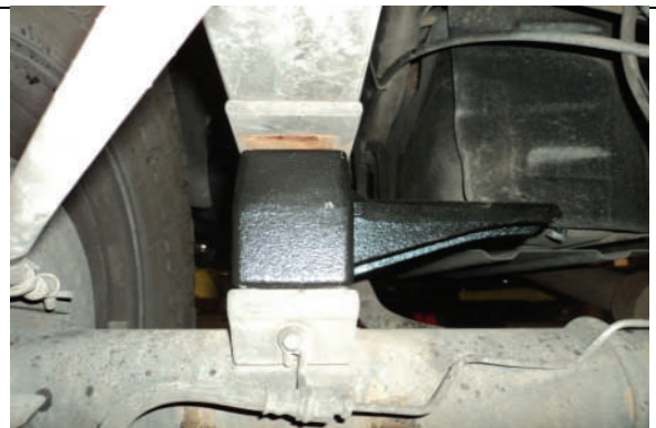
Remove OE axle block and replace w/ new lift block.
