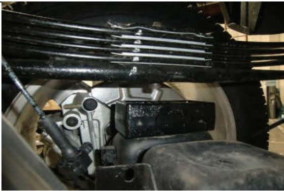
Note slight taper on block, shorter end towards front of truck
