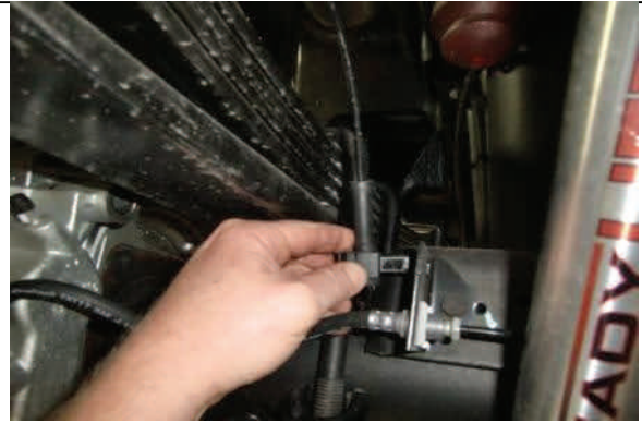
Release ABS clip from bracket on axle.
