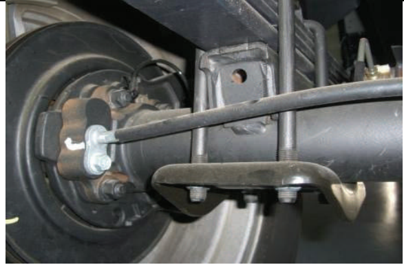
Locate rear leaf spring mount over axle, support axle w/ jack
