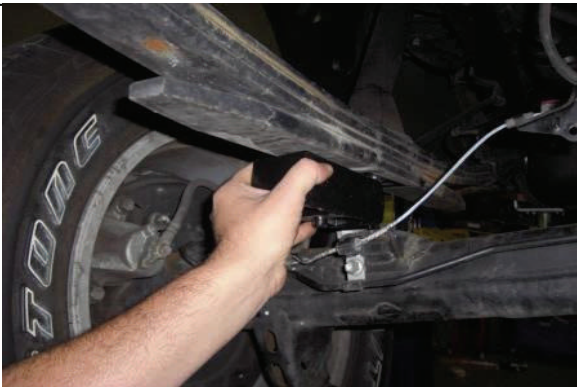
Lower axle enough to install lift block, place and raise axle
