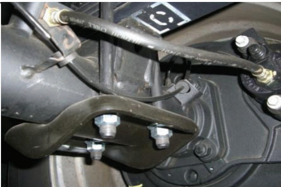
Check center pin alignment and tighten hardware to spec.
