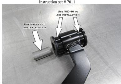
Figure 2: bushing and crush sleeve installation
