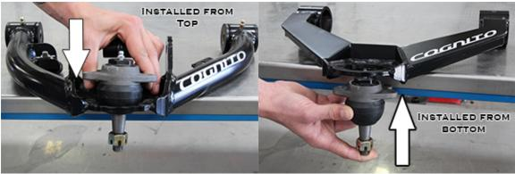
Figure 1: ball joint installation
