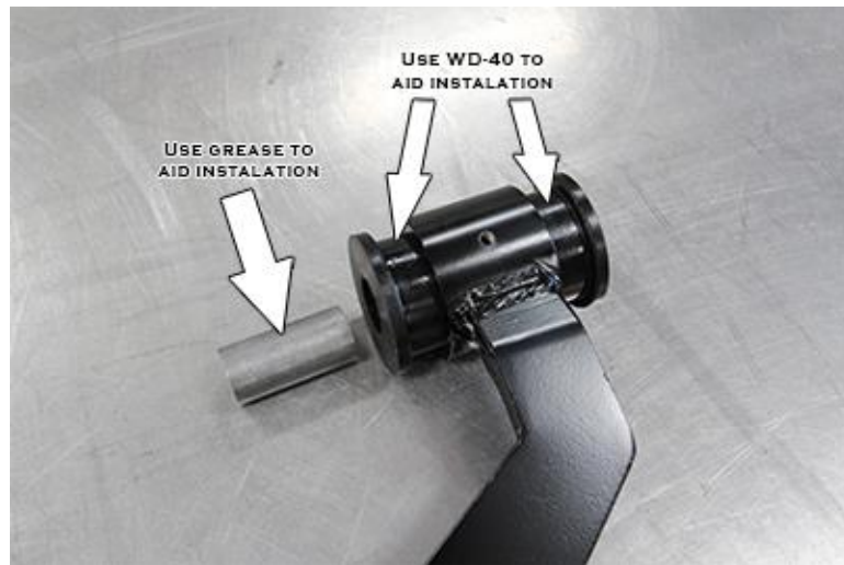
Figure 1: bushing and crush sleeve installation
