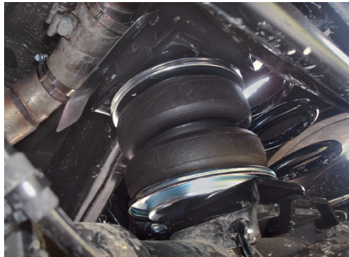
fig. F.3 Inside, rear of axle view of passenger's side installation.
