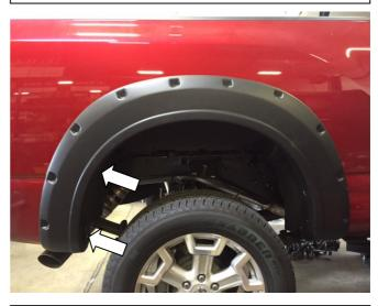
**STEP 12:** Place Fender Flare on vehicle, ensure the slots in the Fender Flare align with the holes in the wheel arch from the previously removed factory screws. Using #2 Phillips head screwdriver re-install the previously removed (2) screws through slots in Fender Flare.
