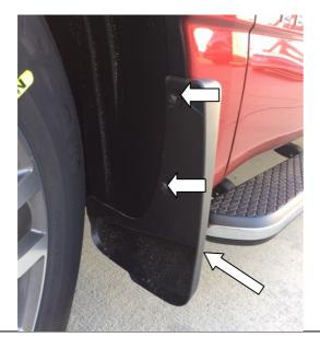
**STEP 5:** For vehicles equipped with factory mud gaurds. Remove (3) retaining screws to remove mud guard. Store mud guard in a safe place, it will not be re-used for Fender Flare installation. Reinstall screw in underside rocker panel area and retain (2) remaining screws from inner wheel arch for Fender Flare Installation.
