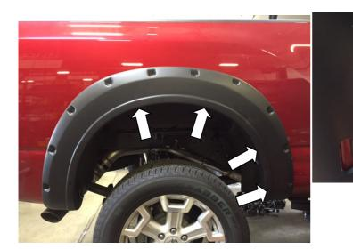
**STEP 13:** Install the provided U shape metal clips in the (4) remaining slot locations in the Fender Flare. Ensure that positive pressure is applied on the Fender Flare to the vehicle fender when installing clips. Slide the clip over the Fender Flare and the inner lip of the wheel arch ensuring that the barb in the clip locates in the slot of the Fender Flare. Ensure all fixing points are tight and secure and that the rubber seal is flush neatly against the vehicle body.
