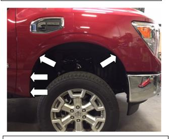
**STEP 6:** Place Fender Flare on the vehicle into the position of best fit. Note where (4) slots in Fender Flare correspond with existing screws / fixing points in the wheel arch. Remove Fender Flare. Remove any existing vehicle screws in locations as shown with #2 Phillips head screwdriver. Maintain screws for re-installation.
