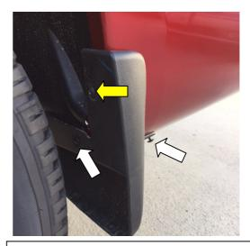
**STEP 10:** For vehicles equipped with factory mud gaurds. Remove (3) retaining screws to remove mud guard. Store mud guard in a safe place, it will not be reused for Fender Flare installation. Reinstall screws in underside rocker panel and innermost wheel arch area retain remaining uppermost screw for Fender Flare Installation.
