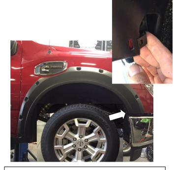
**STEP 8:** Install the provided U shape metal clip at the (1) remaining slot location in the Fender Flare. Ensure that positive pressure is applied on the Fender Flare to the vehicle fender when installing clips. Slide the clip over the Fender Flare and the inner lip of the front bumper fascia ensuring that the barb in the clip locates in the slot of the Fender Flare. Ensure that the rubber seal is flush neatly against the vehicle body.
