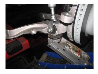
Reattach the lower control into it original location using the o.e bolts and cams.
