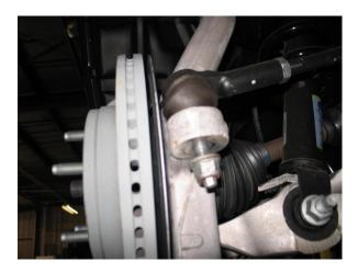
**3a**. Remove plastic clip holding the ABS sensor to the spindle.
