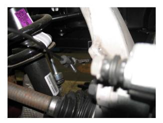
**3b.** To be able to install the Belltech Lift Strut, the lower control arm bolts to the frame must be removed. The lower control arm can then be lowered from those positions. Attached to the bolts are the **alignment cams**. Please take the time to **mark the position** so they can be re-installed in the same position. With a floor jack holding the bottom of the spindle, remove the bolts and lower the lower control arm.
