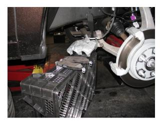
**2c**. Remove steering arm (tie rod) from spindle.
