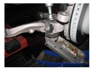
**3a.** Now you can remove the lower strut bolt and the upper mounting nuts.
