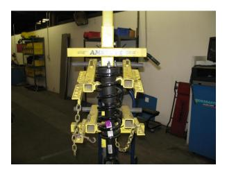
Before disassembling the strut mark the position of the top mount in relationship to the lower bolt hole. Using a spring compressor, compress the spring to remove the pre-load of the spring from the strut. Using the correct tools remove the top mount from the strut. We do not recommend using power tools. Now disassemble the strut and release the spring tension, be sure to remember the order the components are removed.
