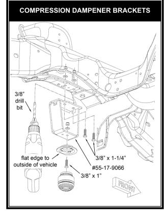
□□ Press the factory compression dampener back into the mounting cup.
