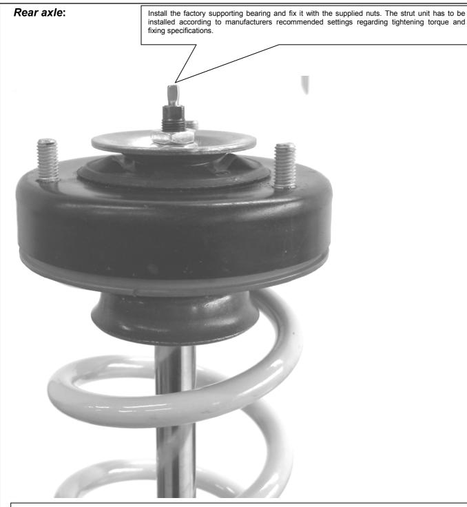
Use the standard additional spring (Elastomer) and the dust cover. This part has to be in perfect condition, otherwise it has to be replaced.
