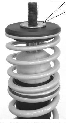
Attach the factory dome bearing and fix it with supplied stop nut. Tightening torque is 60 Nm (44ft-lb). For vehicles with EDC and/or 8 cyl. Motors, additional add on parts from the manufacturer may be necessary:
