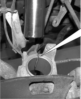
After you have completed installation of the suspension, check the clearance of the wheels/tires to the front suspension system. The minimum clearance at the narrowest point may not be less than 5 mm (0.2 inch). If the wheel/tire does not meet this minimum measurement, TUEV approved wheel spacers may be necessary.
