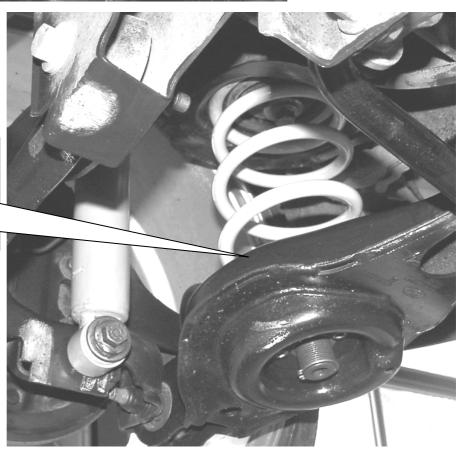
Unless there is no bump stop please use the standard bump stop. The standard bump stop has to be in a good condition, otherwise it has to be replaced.
