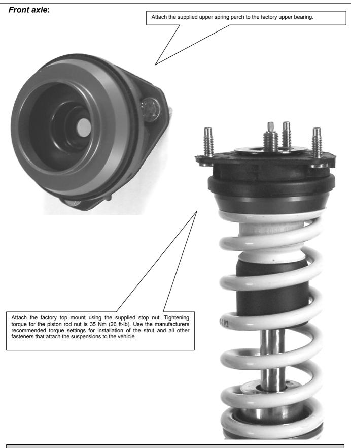
After you have completed installation of the suspension, check the clearance of the wheels/tires to the front suspension system. The minimum clearance at the narrowest point may not be less than 5 mm (0.2 inches). If the wheel/tire does not meet this minimum measurement, TUEV approved wheel spacers may be necessary.
