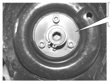
Disassemble the rear height adjustment perch from the mounting plate loosening the 3 bolts and the snap ring). Attach the height adjustment perch to the transverse control arm and fix it as shown on the picture. Tightening torque of the bolts 10 Nm (7 ft-lb).
