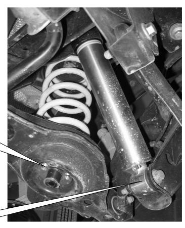
Please install the damper unit to manufacturers recommended settings regarding tightening torque and fixing specifications.
