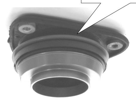
Attach the factory top mount using the supplied stop nut. Tightening torque for the piston rod nut is 35 Nm (26 ft-lb). Use the manufacturers recommended torque settings for installation of the strut and all other fasteners that attach the suspensions to the vehicle.
