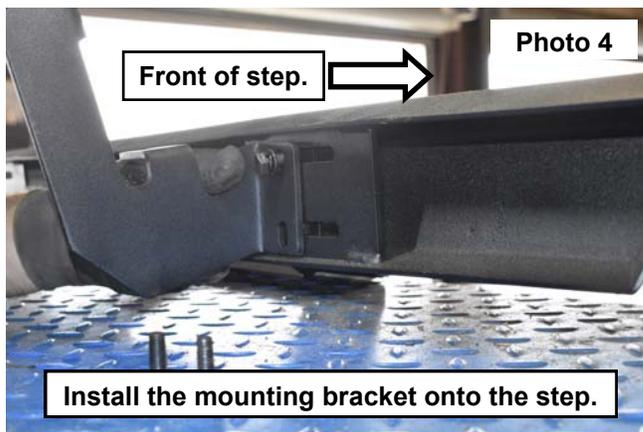
5. Install the 2 remaining nut plate and mounting brackets onto the drivers side step using the supplied 8mm hardware.
