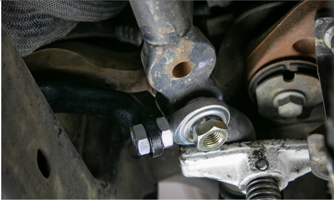
Figure 9: Idler Arm Bracket Installed
