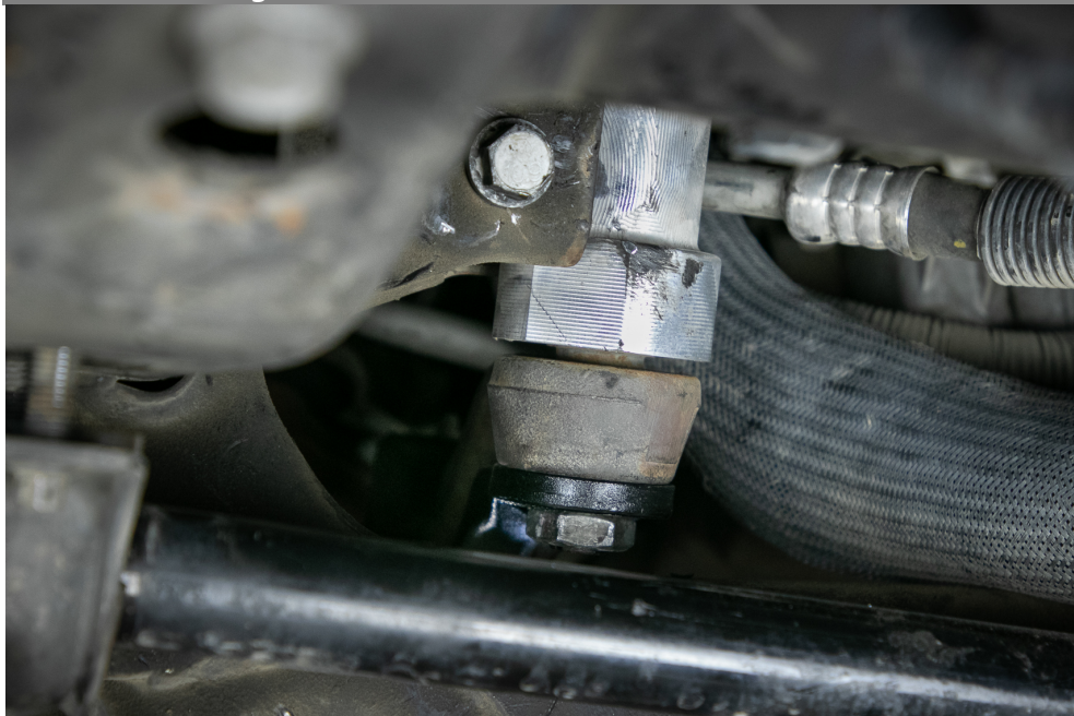
Figure 10: Idler Pivot Reinstalled into Frame
