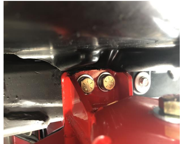
Figure 13: Fuel Tank Shield Trimmed
