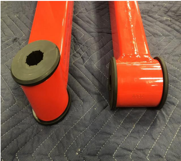
Figure 28: Traction Bar Bushings Installed
