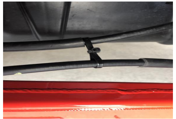
Figure 22: Brake Cable Ties
