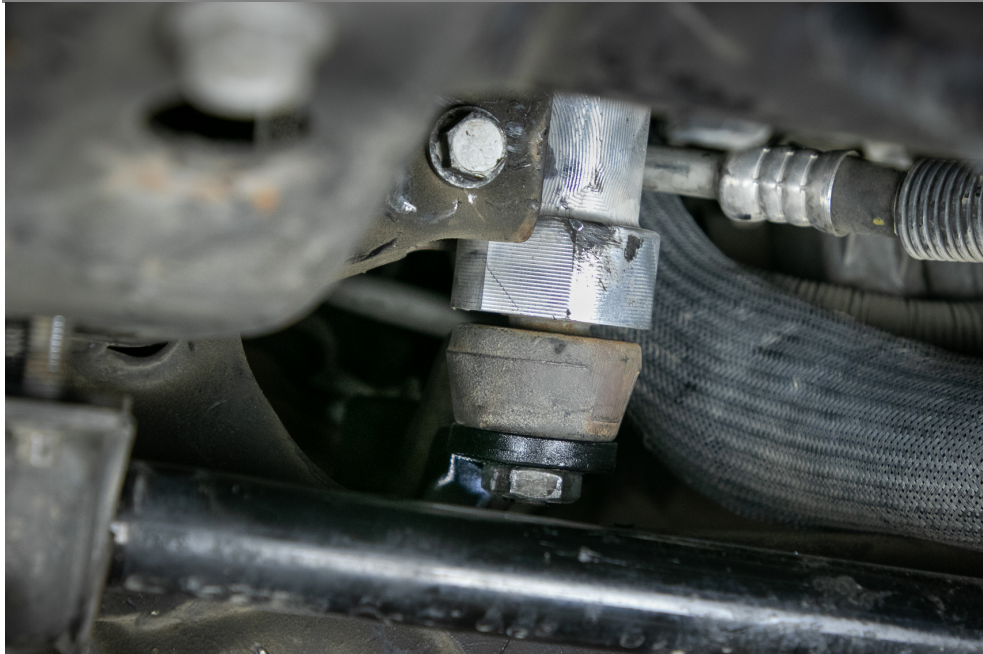
Figure 10: Idler Pivot Reinstalled into Frame
