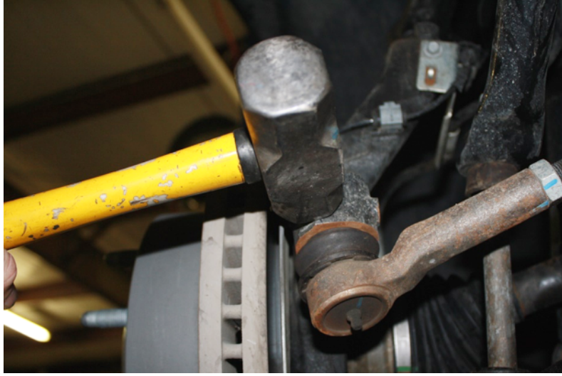
Figure 6: (OPTIONAL) Remove Tie Rod from Passenger Spindle
