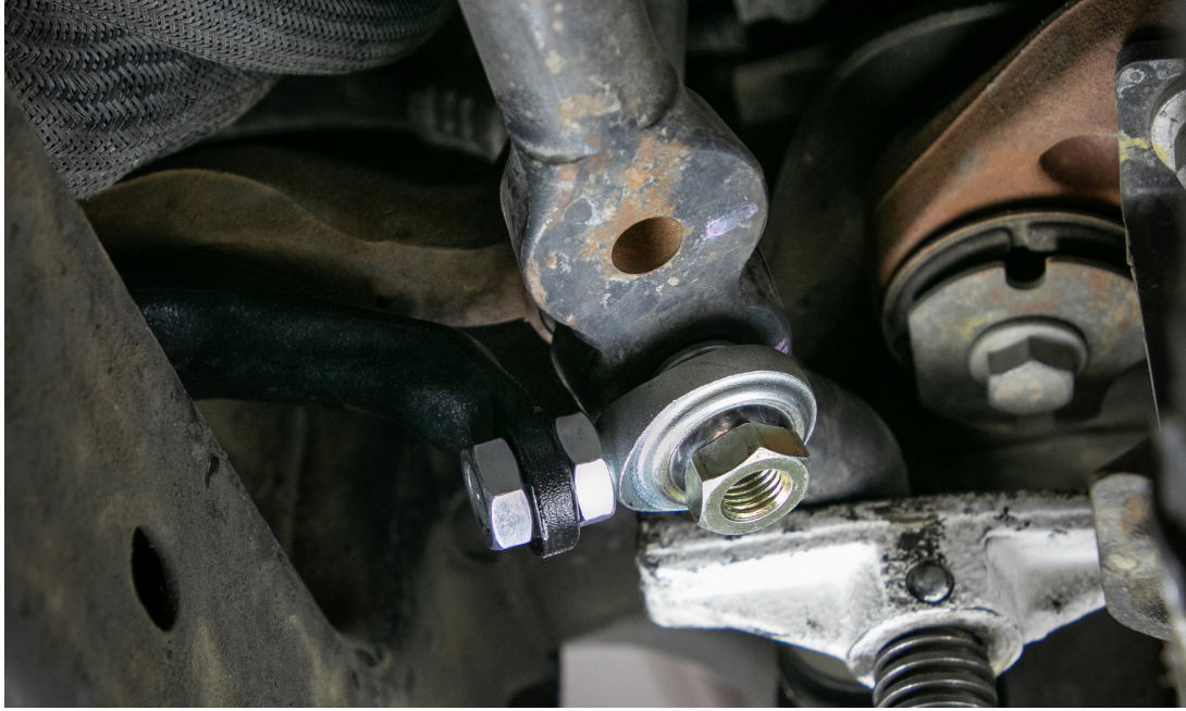
Figure 9: Idler Arm Bracket Installed
