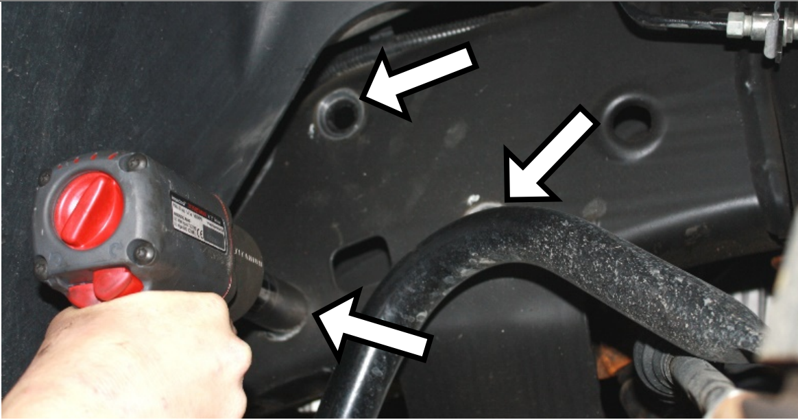
Figure 5: Removing Bolts Holding Steering Box to Frame
