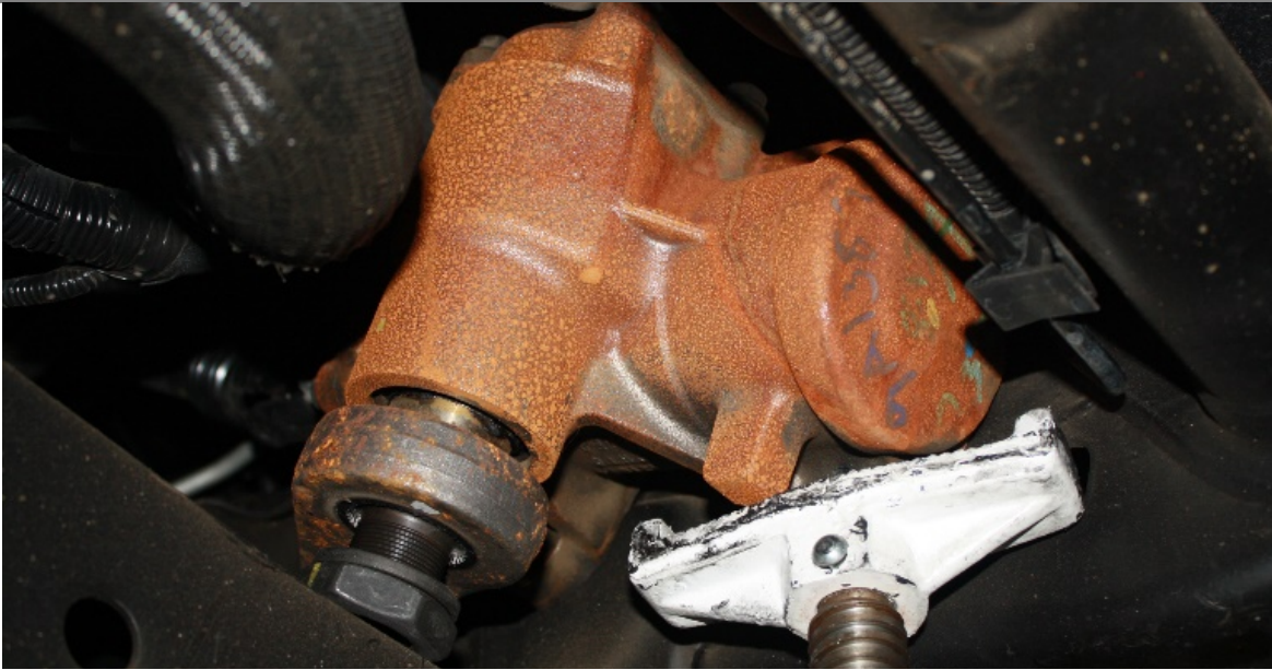
Figure 4: Support the Steering Box with a Jack
